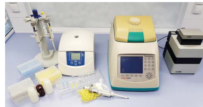
Fig. 1: The needed laboratory equipment are a centrifuge, a PCR-cycler and the gel-electrophoresis device E-CUBE.
